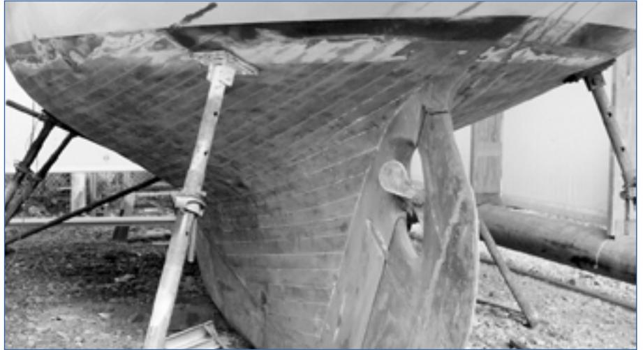
Hull taken back to bare timber. Some seams repaired above and below waterline (1988)
