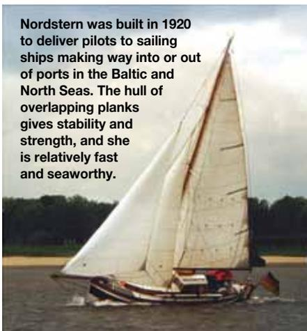
**Nordstern was built in 1920 to deliver pilots to sailing ships making way into or out of ports in the Baltic and North Seas. The hull of overlapping planks gives stability and strength, and she is relatively fast and seaworthy.**
