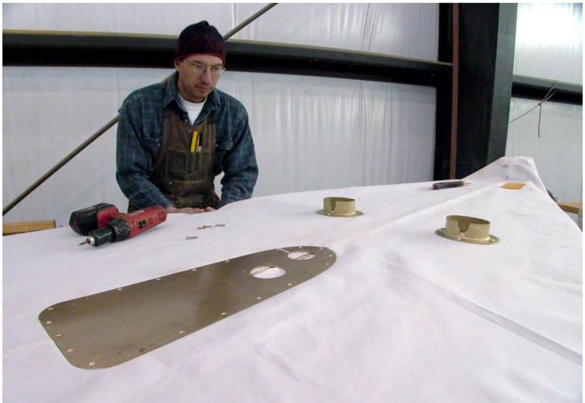
*Shipwright Dave Grizwold test fitting the hardware into the cloth in preparation for final laying of the material*
