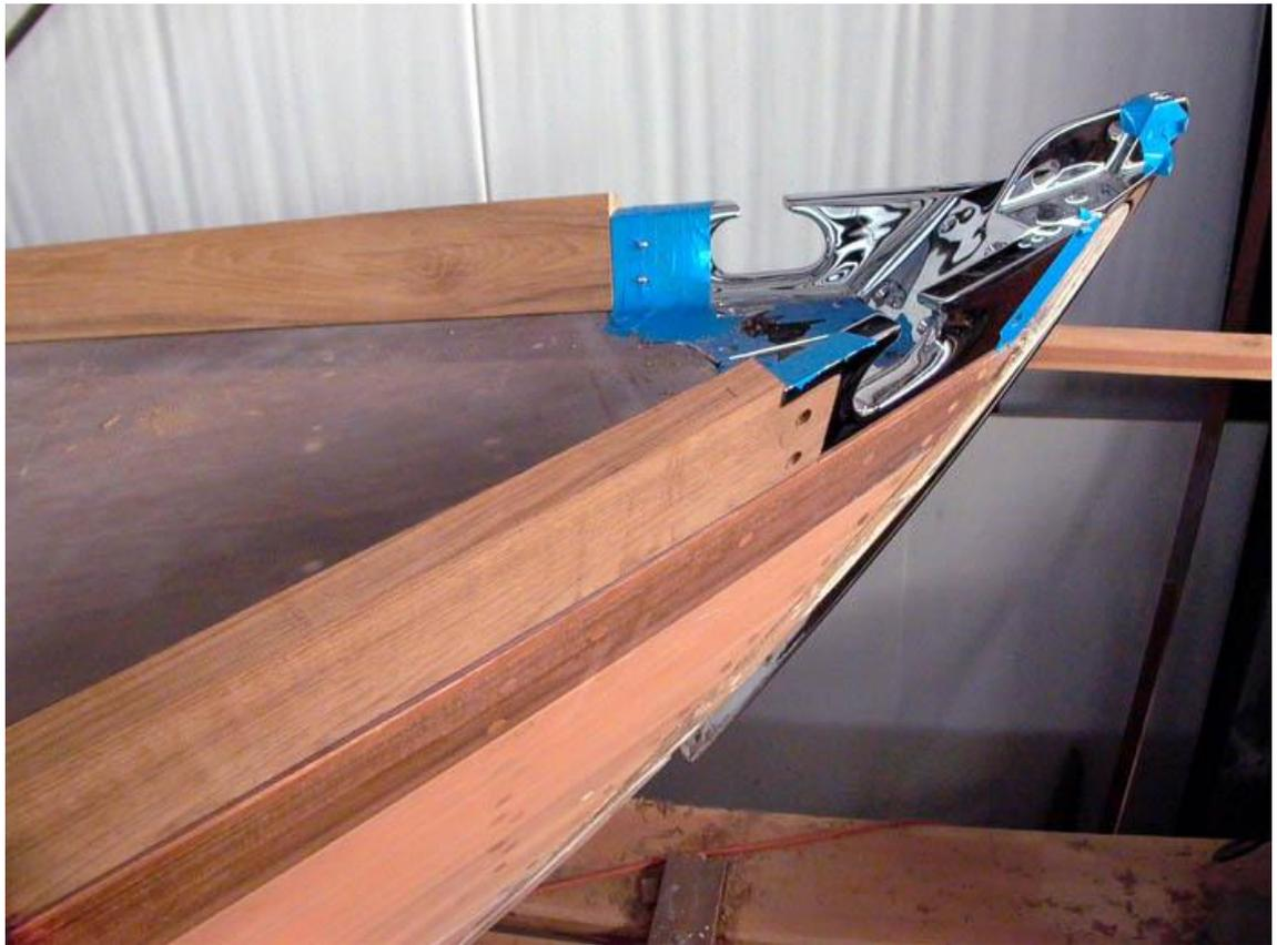
*The prepared deck can be seen here with the toe rails fit into the original Nevins hardware.*
